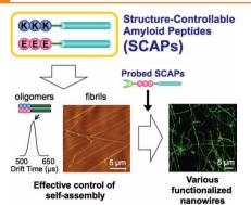
Straightforward preparation of various functionalized or inorganic nanowires can be achieved by a very simple method based on mixing structurally related modified amyloid peptides, which allows effective control of self-assembly. The peptides contain three-amino-acid-residue units that provide remarkable control during the entire self-assembly process, starting from a small oligomer up to the macroscopic fibril level.
