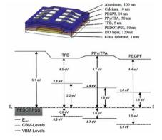
A conceptual study on triple-layer PLEDs fabricated by successive solution based deposition of multiple polymer layers without extensively redissolving of existing layers is shown. Ultraviolet photoemission spectroscopy (UPS) measurements of the triple-layer assembly reveal a favorable energy level alignment at the respective material interfaces resulting in a charge carrier confinement in the emitting layer, thus enhancing maximum luminance and luminous efficiency values.
