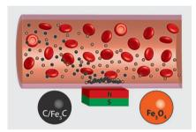
The responsiveness to external magnetic fields is a critical parameter for the successful application of nanomagnets in biomedicine, as fast and complete magnetic separations are essential. Here, the superior separation performance of strongly magnetizable carbon-coated cementite nanoparticles over magnetite nanomagnets from stagnant/flowing human blood is shown. Beyond, a robust quantification approach for iron-based nanomaterials in iron-rich matrices is presented.
