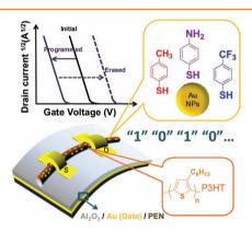
Novel flexible nonvolatile trandevices based sistor memory on the electrospun nanofiber of poly(3hexylthiophene):surface-modified nanoparticles show a low voltage operation (±5 V), large threshold voltage shift (3.5-10.6 V), long retention times (>104 s), and good endurance properties (>100 cycles) regardless of mechanical bending stress.
