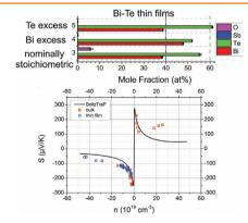
Wavelength-dispersive X-ray spectrometry (WDX) is applied to Bi<sub>2</sub>Te<sub>2</sub> thermoelectric thin films for accurate chemical analysis. The antisite densities can thus be measured and this can be used to control the charge-carrier densities. The transport properties are compared with solutions of the linearized Boltzmann transport equation. For sputtered films, the argon concentration, which is relevant for phonon scattering, is measured.
